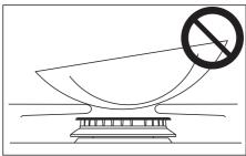
Avoid using unstable and misshapen pans that may tilt easily and pans with a very small base diameter e.g. milk pans, single egg poachers. The minimum pan diameter recommended is  $4^{3}/_{4}$ ".
